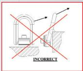
5. The use of free fit spacers should not be used between the hoist ring and the mounting surface. This will reduce the working capacity of the device. See below:
